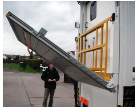
Standard 'Ratcliff' passenger tail lift
