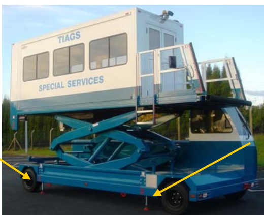
2 hydraulic stabilizers at each side
