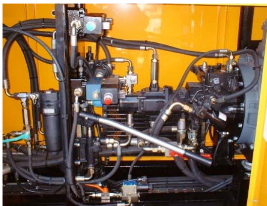
Hydraulic Components including Emergency facilities
