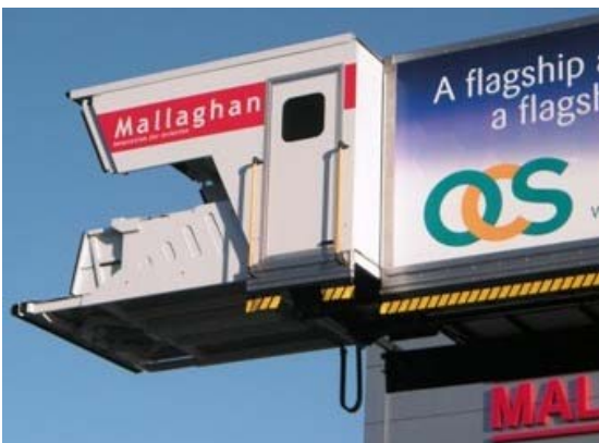
Platform and Operator cabin traversed to the left
