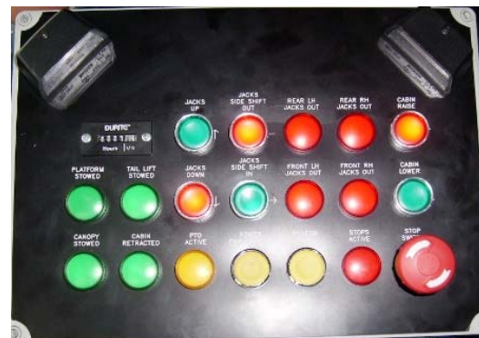
Standard Driver's Cab Control Panel
