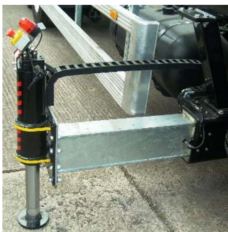
Hydraulic stabilizer with telescopic outrigger
