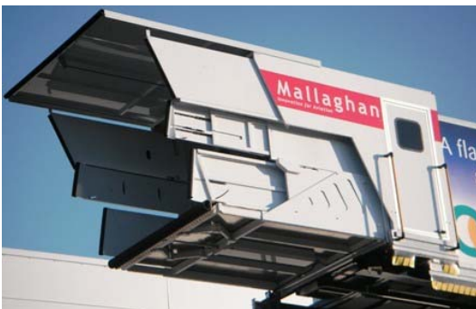
Platform floor, roof and side panel extensions fully out
