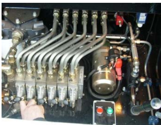
Hydraulic Valves with manual override
